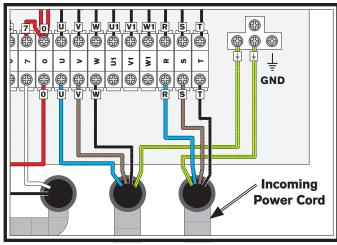
Figure 52. Power connection wiring.
